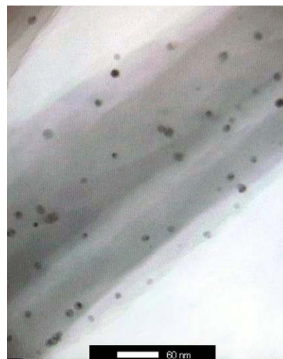
Fig. 5. TEM images of the CA nanofibers containing 0.5 wt% \text{AgNO}_3 after irradiation with UV light at 365 nm for 240 min. The scale bar corresponds to 60 nm.
