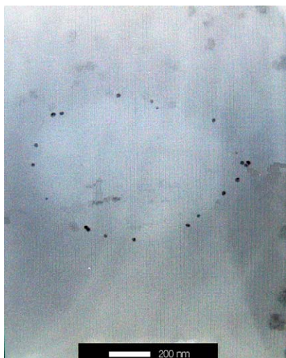
Fig. 6. Cross-sectional TEM images of the CA nanofibers containing 0.5 wt% \text{AgNO}_3 after UV irradiation for 240 min. The scale bar corresponds to 200 nm.
